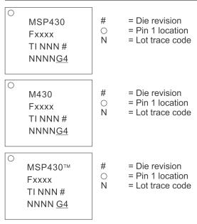
NOTE: Package marking with "TM" applies only to devices released after 2011.
